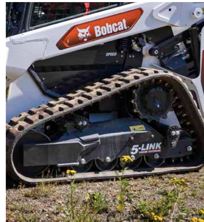
5-link torsion suspension system
